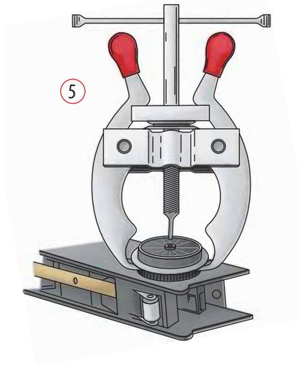
With one hand, make sure the puller clamps are held against the gear wheel teeth. (Fig. 5.) With the other hand, begin to turn the threaded bolt until it comes in contact with the end of the axle. (Fig. 6.) Tighten the wheel puller slowly. The wheel should pop off the axle with only moderate pressure. If it doesn't, remove the wheel puller and try soaking the locomotive wheels in penetrating oil overnight.
